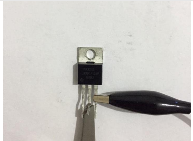
Figure 136: Channel1 Probe Used for Drain - Source Measurement
