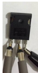
Figure 145: Sample of a Defective N Channel FET
