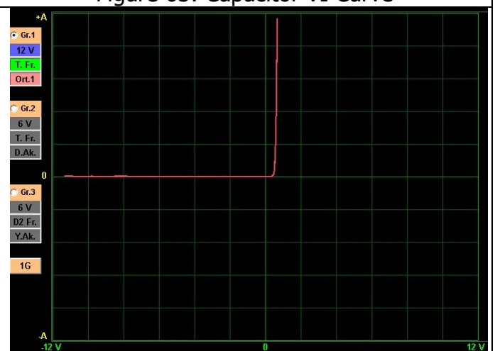
Figure 65: Diode VI Curve
