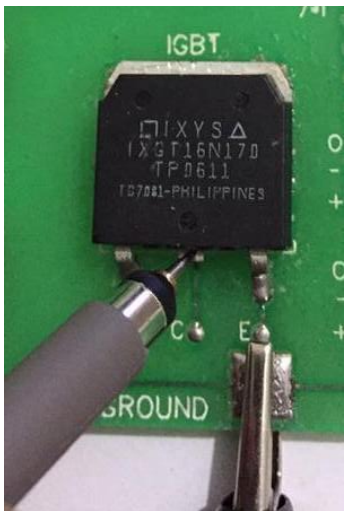
Figure 152: Channel1 Probe Used for Collector - Emitter Measurement
