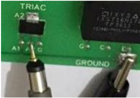
Figure 171: Channel1 Probe Used for Anode2 - Anode1 Measurement
