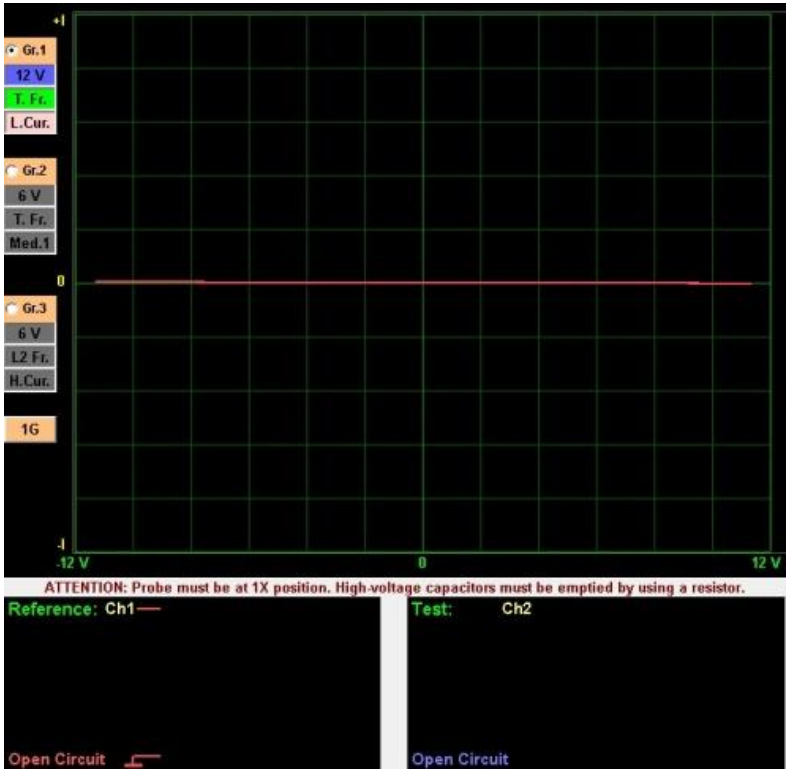
Figure 161: Gate (+) Anode (-) VI Graph
