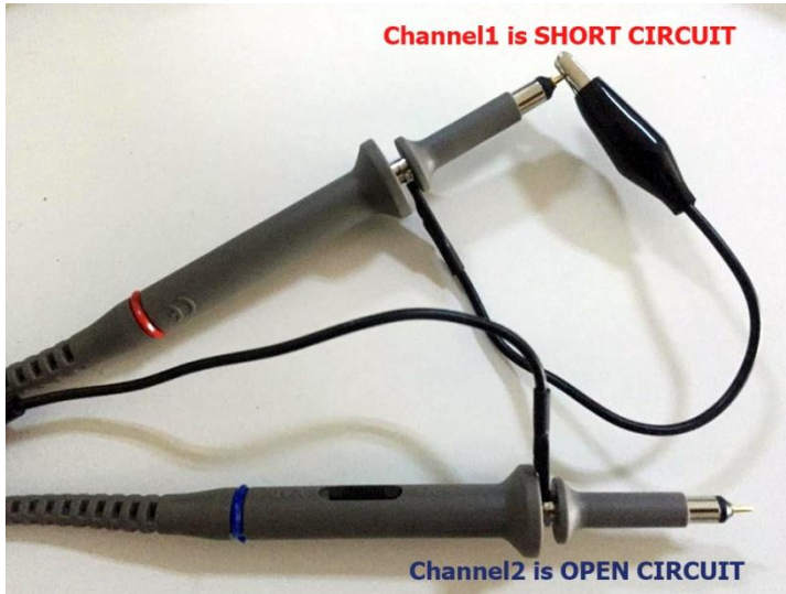
Figure 56: Short Circuit (Channel1) - Open Circuit (Channel2)
