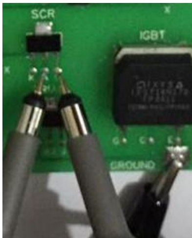
Figure 164: Channel1 (+), Channel2 (+), COM (-) Thyristor Test
