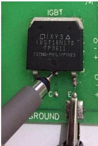
Figure 150: Channel1 Probe Used for Collector - Emitter Measurement
