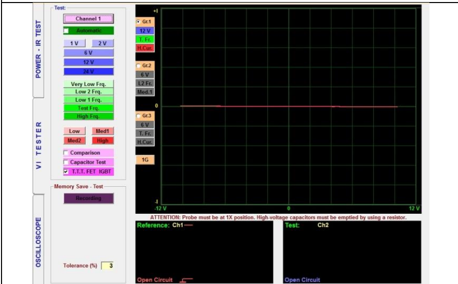
Figure 151: Collector (+) Emitter (-) VI Graph
