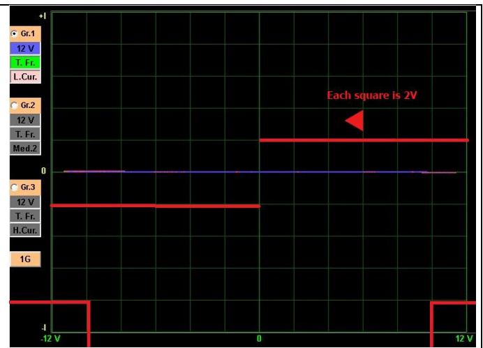
Figure 60: If the Test Voltage 12V, Each Square Represents 2V.
