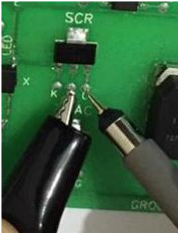
Figure 158: Channel1 Probe Used for Gate - Cathode Measurement
