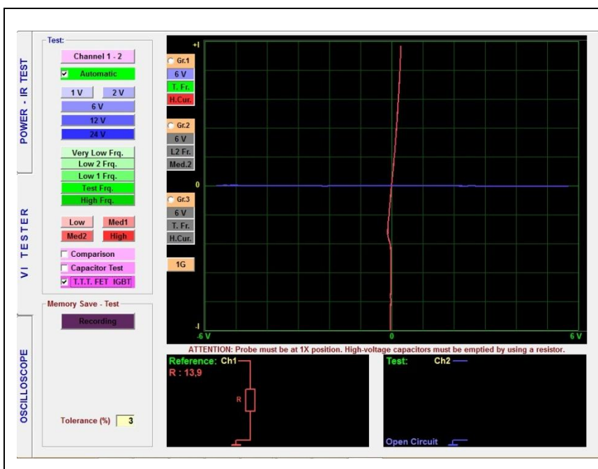
Figure 144: Sample of a Defective P Channel FET
