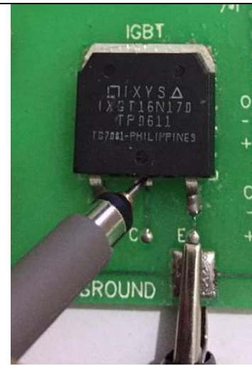
Figure 154: Channel1 Probe Used for Collector - Emitter Measurement
