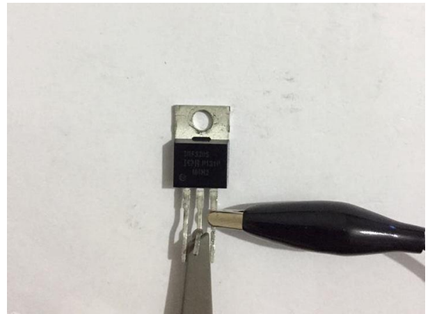
Figure 134: Channel1 Probe Used for Drain - Source Measurement
